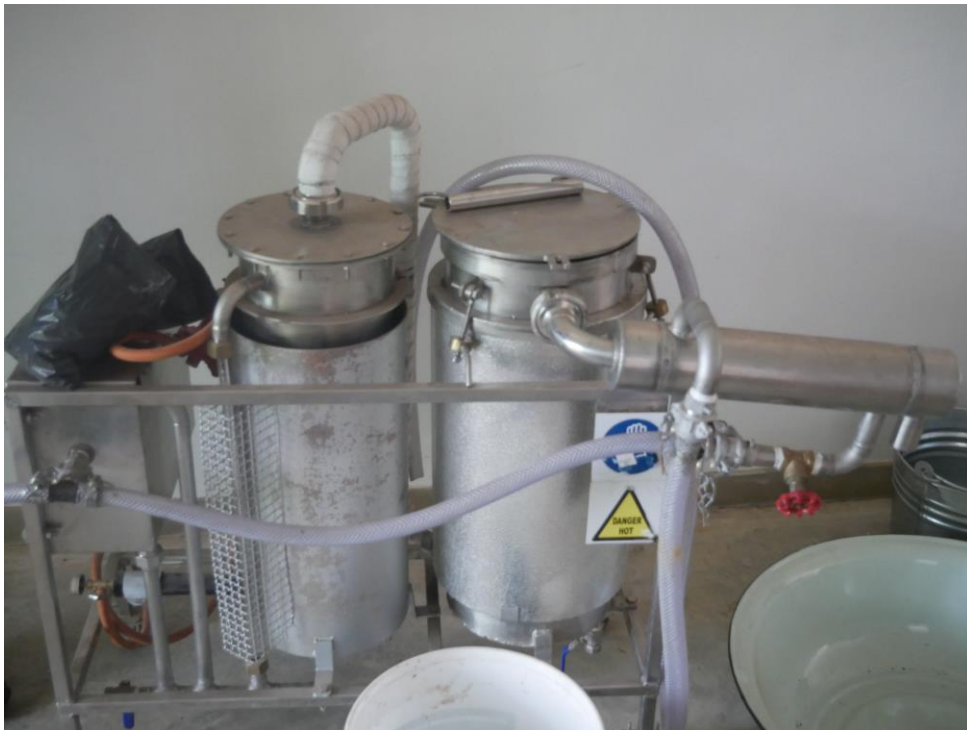
Figure 3: The smaller distillation equipment (10kg) for tester production of oils from plant materials
