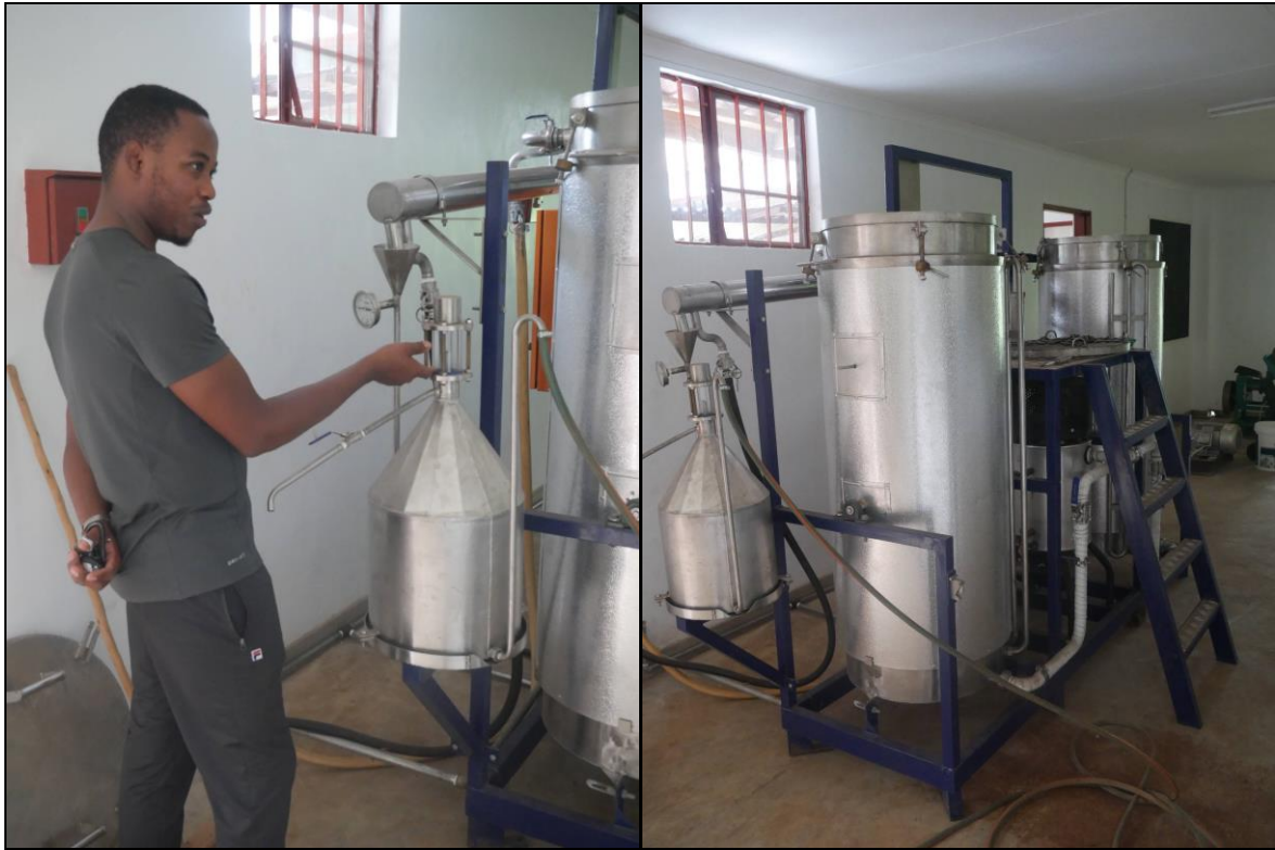
Figure 2: The larger distillation equipment (100kg) with project manager, Ibrahim Mitole, explaining how the oils are produced ( left )
